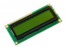
The following shows a typical usage where d4 to d7 are connected to pins GP2 to GP4 on the PicoMite, rs is connected to pin GP6 and en to pin GP7.
